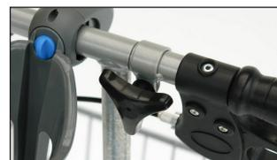
**Photo C.** Handbrake lever on Scooter
